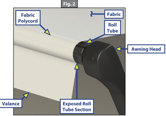
**NOTE:** The awning fabric should always be above the roll tube. However, if the EXTEND switch is engaged too long or EXTEND is hit inadvertently instead of RETRACT, the awning will roll up backward. This is not a defect. To correct the fabric orientation, press the RETRACT button. The awning will then extend to its correct orientation and normal operation can resume.
